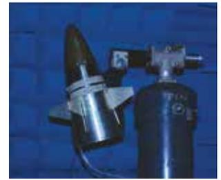
*XM 982 Nosecone with Dual-band L1-L2 GPS Antenna Array*
