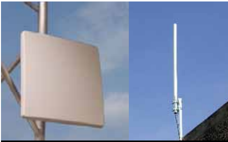
Flat panel and omnidirectional antennas for smart grid remote monitoring and control
