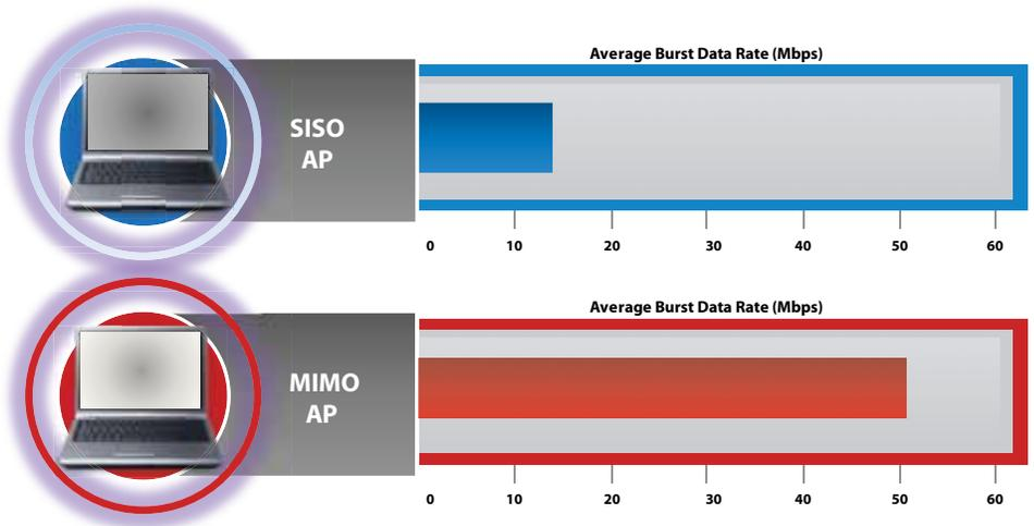
In MIMO 2x3 Receive Diversity Systems, smart antennas use spatial diversity technology to improve signal-to-noise ratio. For example, if the receiver has more antennas than spatial streams (in a 2x3 system two antennas transmit while three antennas receive) the third antenna can add diversity to the receiver end, improving system robustness through longer distances at given speeds.
